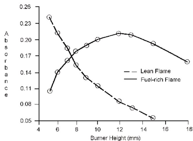
Figure 1. Flame profiles of calcium absorbance in various flame conditions (serum samples).
