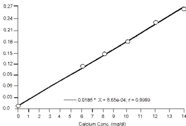
Figure 2. Linearity of the calcium reference method using a fuel lean air-acetylene flame.
